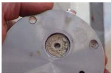
Fig. 11. Sulfur on HAG Probe Particulate Filter After TGTU Process Upset
