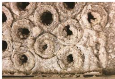
Fig. 5. Ammonia Salts on Process Condenser Tube Sheet (courtesy of Sulphur Experts)
